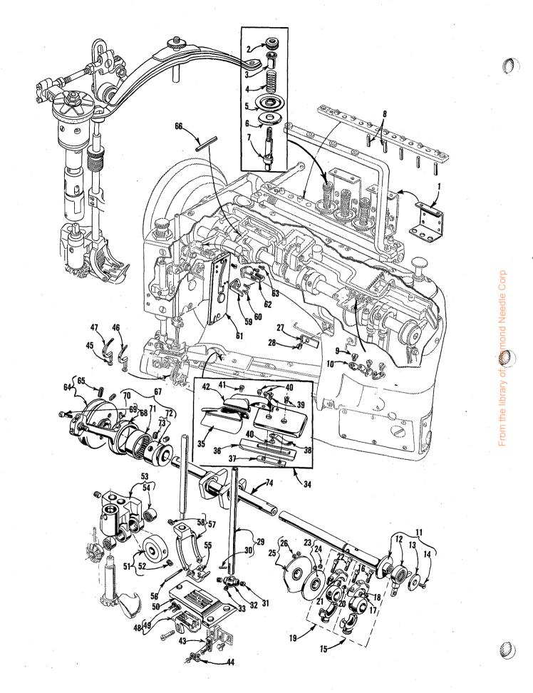
The parts illustrated on pages 8 and 10, and described on this page and page 11 epresent the parts that are used on Style 35700 CP, but not used on Style 35800 DQ.
